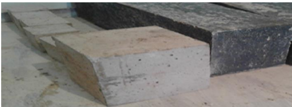
Figure 2: Samples made of geopolymer concrete based on zeolite.
