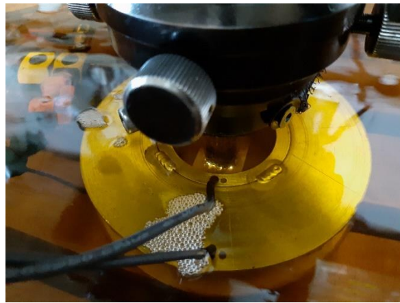
Figure 10: Image of EDM Machining with the assisted of magnetic field system designed.
