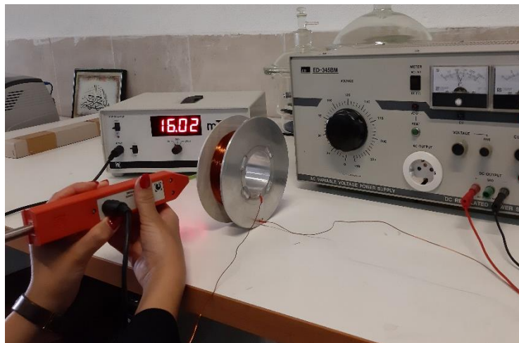
Figure 9: Image of the coil performance checking in laboratory.
