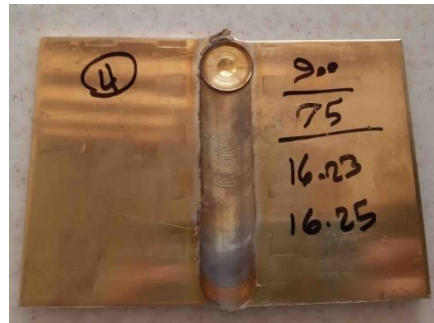
Fig. 3: Crown side of the FSW No. 4.
