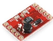
Fig. 4: Small energy storage board with using LTC3588-1 regulator.
